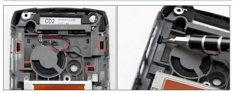
• Press in the four black clips using a spudger to pop off the upper-back cover.
