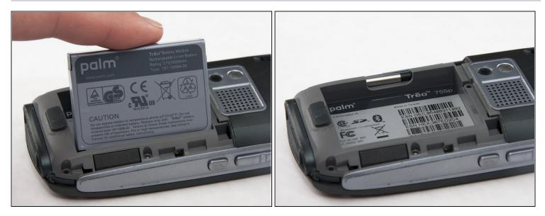
• Remove the battery by lifting up on one side.
