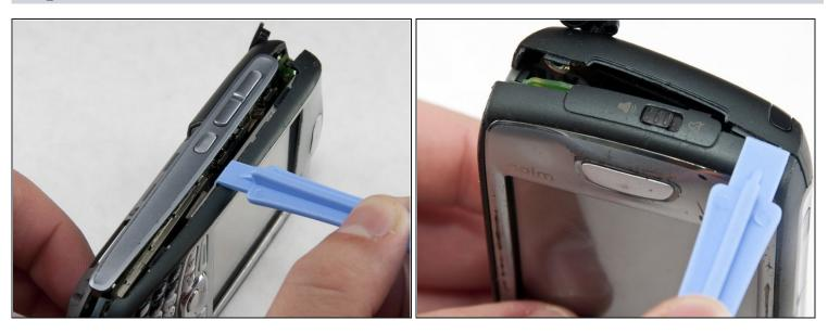
• Use the plastic opening tool to pry open the device. Start on the volume control side (left side of the screen) and work your way up along the edge and across the top.
