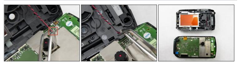
• Using <u>tweezers</u>, squeeze the plastic head of the black and red wound wire cable. This will detach the cable from the circuit board and fully separate the two halves.
