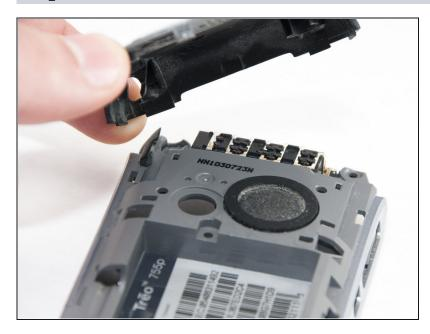
• Lift off the top of the back cover from the phone frame.
