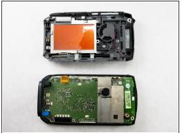
Using tweezers, squeeze the plastic head of the black and red wound wire cable. This will detach
