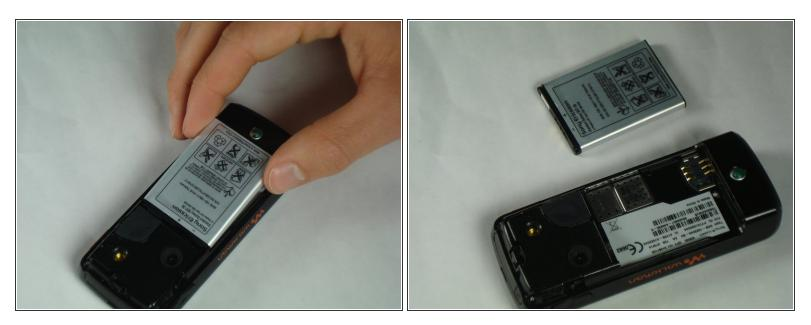
• Pop the battery out of its slot by lifting it up.
