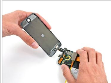
Remove the display assembly from the iPod.
