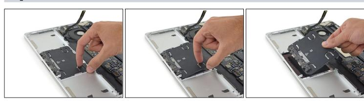
• Lift up and remove the trackpad from the upper case.
