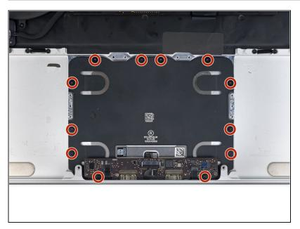
• Remove the twelve 2.4 mm T5 screws securing the trackpad to the upper case.
