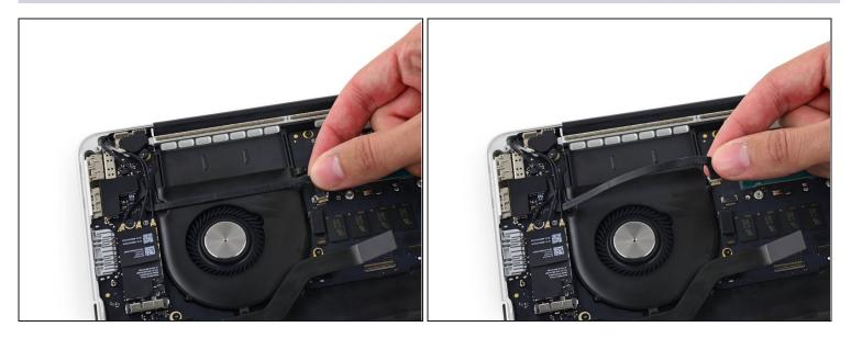
• Peel the iSight camera cable up off the fan housing to fold it out of the way.
