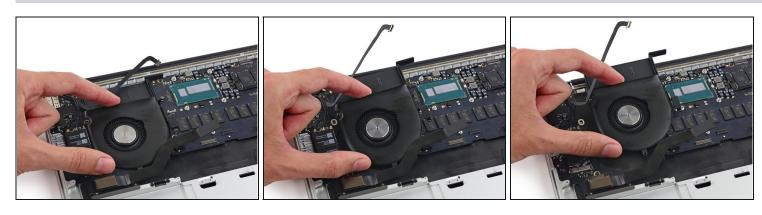
• Lift the end of the fan from the heat sink cavity and pull it up and out toward the hinge of the laptop to remove it.
