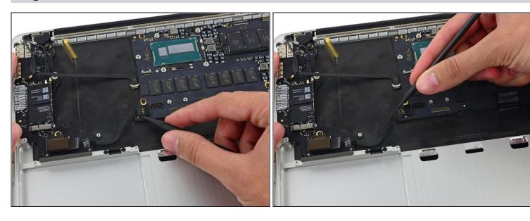
• With the tip of a spudger, push on either side of the I/O board connector to *walk* it out of its socket on the logic board.
