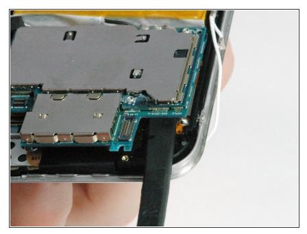
In a similar manner, slide a spudger beneath the logic board where the camera was. Again, don't lift up too far yet as there are still four attached connectors on the bottom of the logic board.
