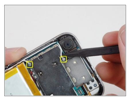
Use a spudger to disconnect the two antenna cables from the communications board. Apple used a small dab of glue on these connections, which may make removing the antenna connections harder.
