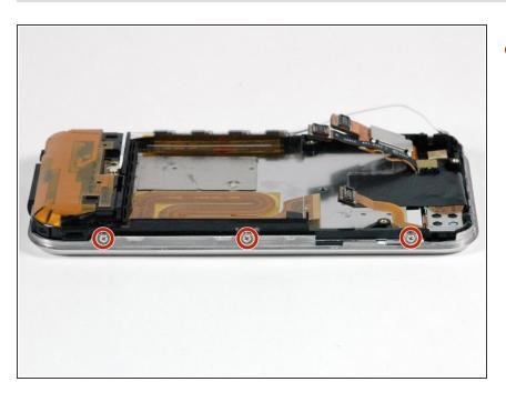
Remove the three Phillips #00 screws securing the front bezel to the iPhone.
