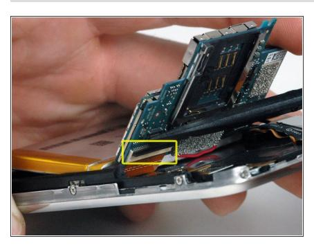
Slide a spudger beneath the black locking bar and pry up to rotate the bar 90 degrees (the bar is already rotated in the picture).
