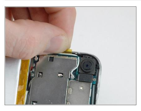
Peel up the orange tape securing the white antenna cable to the side of the iPhone.
