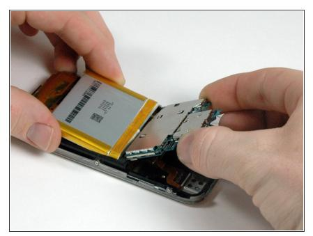
Hold both the battery and the logic board assembly and slide both parts away from the orange antenna and out of the iPhone.
