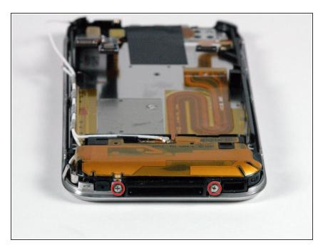
Rotate the iPhone 90 degrees and remove the two Phillips #00 screws from the bottom of the iPhone.
