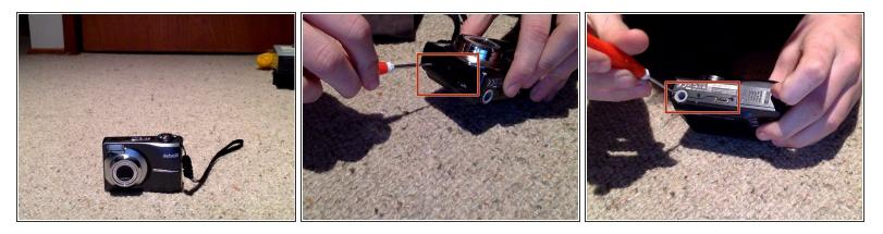
• First you want to remove the 7 Philips Head Screws from the exterior of the camera
