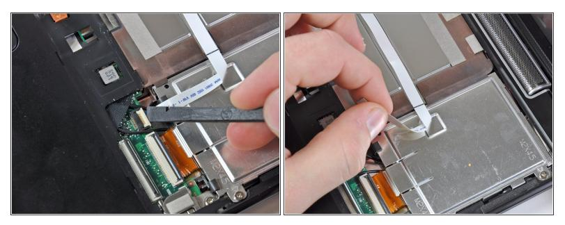
• Use your fingernail or the flat end of a spudger to flip up the retaining flap on the SIM card ribbon cable ZIF socket.
