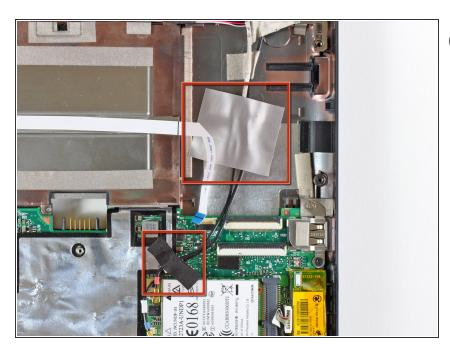
*i* If present, remove the pieces of tape securing the Wi-Fi antenna cables to the upper case.
