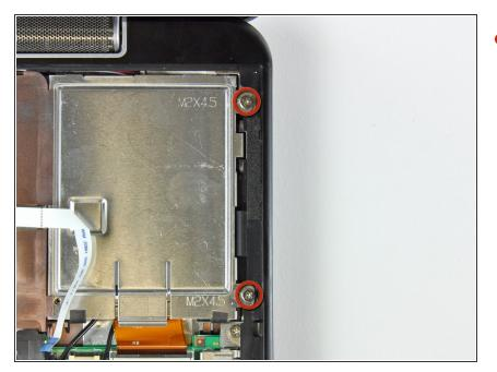
Remove the two 4.5 mm Phillips screws securing the hard drive to the lower case.
