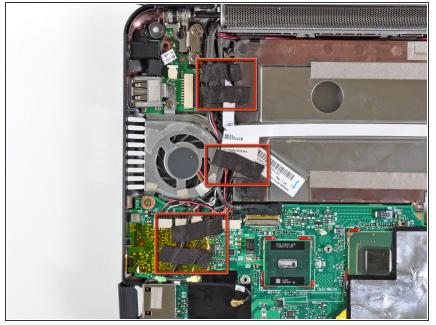
(i) If present, remove the several pieces of black cloth tape securing the cables to the upper case near the fan.
