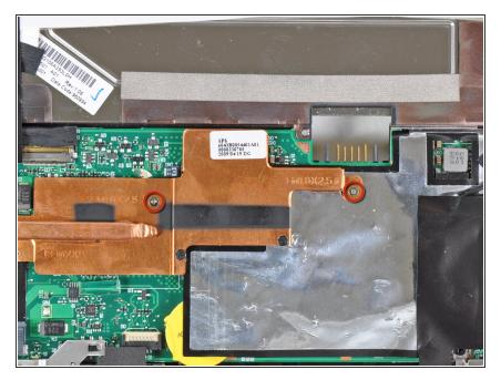
Remove the two 2.5 mm Phillips screws securing the heat sink to the motherboard.
