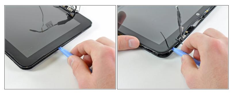
• Finally, use a plastic opening tool to release the retaining clips along the left side and bottom left corner of the display.
