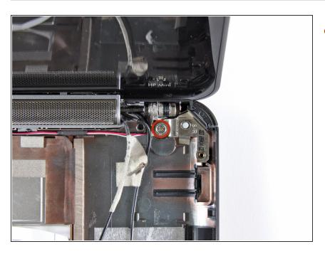
Remove the single 5 mm Phillips screw securing the right display hinge to the lower case.
