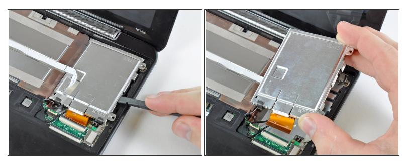
Lift the hard drive up and out of the lower case, being careful not to damage its cable in the process.
