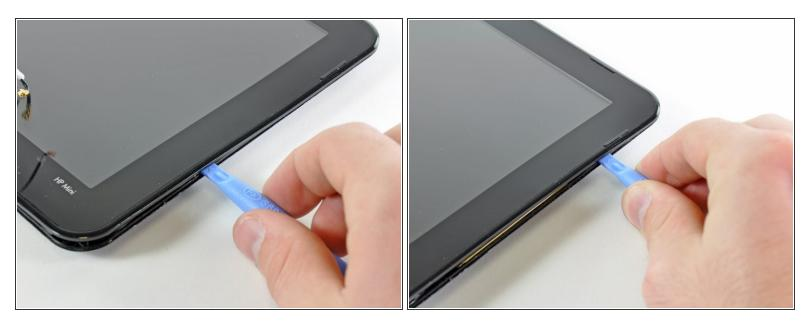
Continue prying to release the clips attaching the front display bezel to the right side of the display's rear section.
