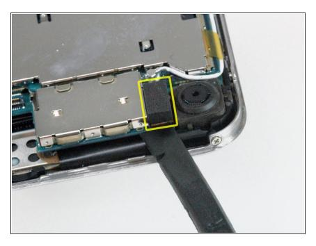
Use a spudger to disconnect the camera connector.
