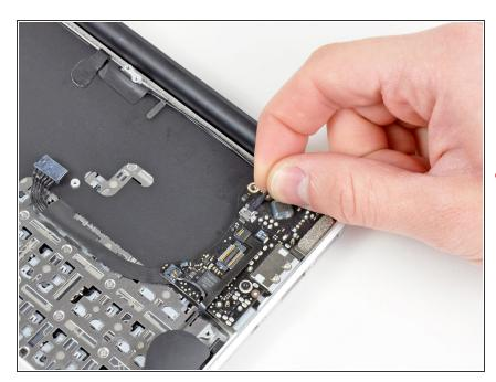
• Pull the camera cable parallel to the face of the I/O board toward the rear edge of the Air to disconnect it from its socket.
