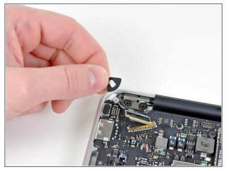
• Remove the small rubber gasket from the corner of the upper case near the display data cable.
