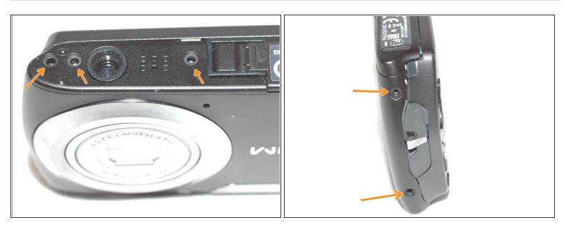
• Remove three screws on bottom and two on the side
