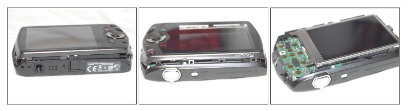
• Carefully lift rear cover with a spudger. Start with bottom side first, then top side.
