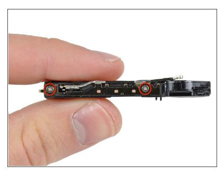
Remove the two Phillips screws securing the antenna to the speaker enclosure.
