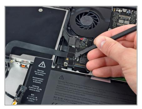
Use the flat end of a spudger to pry the hard drive cable connector up off the logic board.
