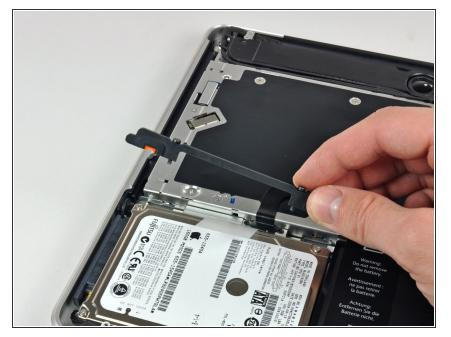
• Lift the the retaining bracket out of the upper case.
