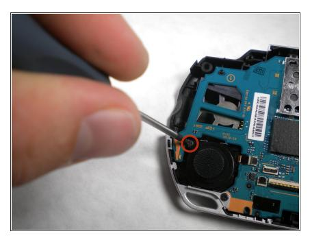
Remove a single Phillips screw securing the analog stick to the PSP 300xc.
