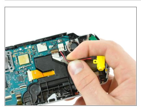
Disconnect the power jack from its connector on the motherboard by pulling it straight out of its socket.
