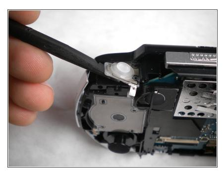
Using the flat end of a spudger, peel the 'L' trigger contact pad up from the case.
