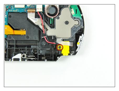
Remove a single Phillips screw securing the power jack to the PSP.
