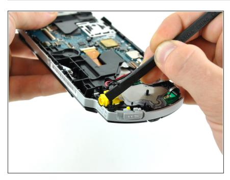
Using the flat edge of a spudger, pry the small black tab away from the power jack to free it from the case.
