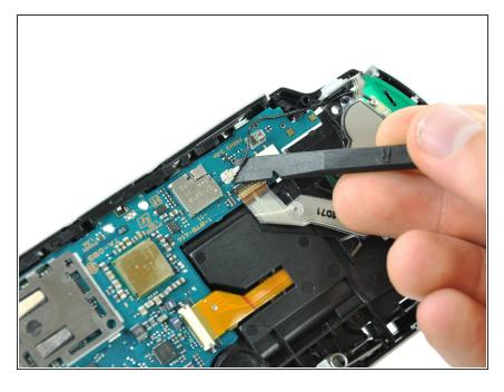
Using the flat edge of a spudger, pry the wireless board cable connector straight up and off the motherboard.
