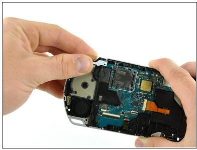
Remove both trigger buttons by lifting them off the PSP 300xc.
