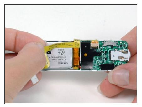
• Carefully peel the yellow USB ribbon up from the battery.
