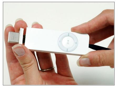
After the USB port comes free, carefully slide it out of its housing. Don't pull it out too far because there's still a ribbon cable connecting it to the logic board.
