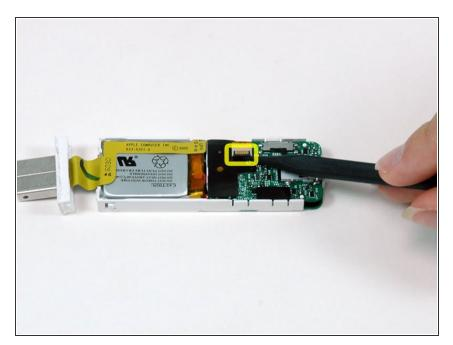
Use a spudger to flip up the black plastic tab holding the USB port ribbon in place. The black tab will
