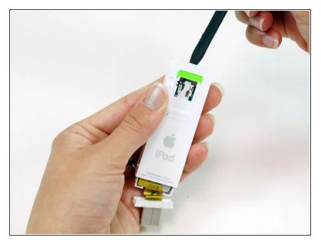
Continue to slide the iPod out of its casing by using a spudger to push on the logic board near the headphone jack.
