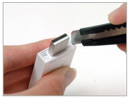
Continue to run the knife around all four edges of the USB port until the glue is released. You may be able to gently wiggle the knife from side to side to help release the glue.
