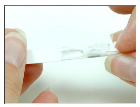
Peel up the translucent tape securing the memory board to the edge of the white plastic framework. It is only necessary to peel up the tape on one side, as the other side will be freed while removing the memory board.
