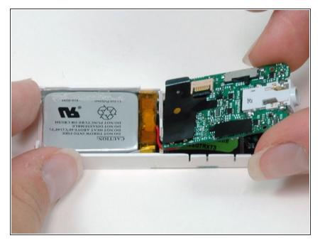
Lift the logic board up to disconnect it from the memory board beneath.
