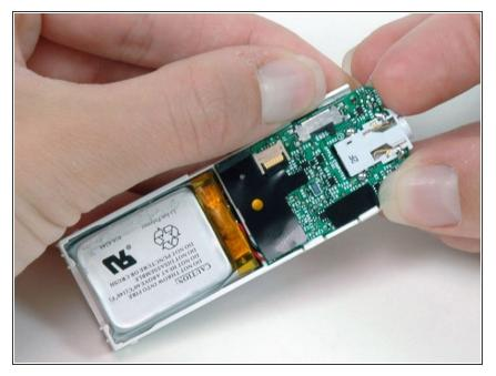
Gently pull back the white plastic framework to free the left edge of the logic board. Pull up on the logic board slightly to prevent the logic board from falling back into place.
