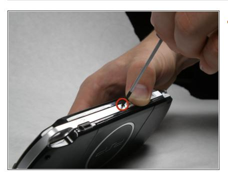
Remove a single screw from the bottom edge of the PSP.
