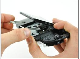
Slide the UMD brace toward the top of the UMD door until the brace disconnects from the door.
