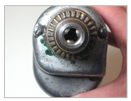
Pull the drill bit free as the jaws loosen.
