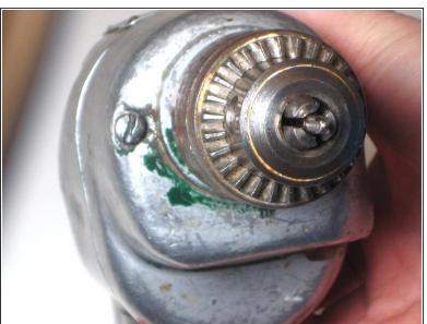
Locate one of the indents in the side of the chuck. Line up the chuck key with this hole and the teeth right below it.
