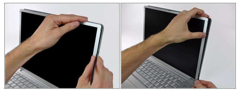
Use a spudger to release the clips along the right edge of the display.
