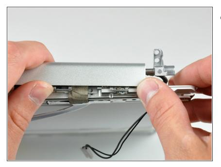
Repeat this process for the other side of the clutch cover. Once the clutch cover is completely free from the clutch hinges, lift it off the front display bezel.
