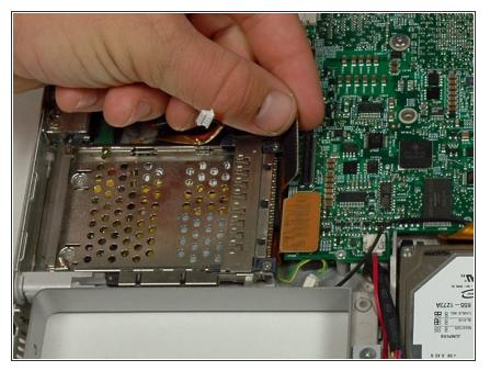
• Disconnect the PC card cable from the logic board.
