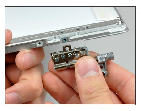
Remove the left clutch hinge from the front bezel.
