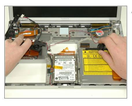
Lift the speaker assembly (including the right speaker) out of the computer.
