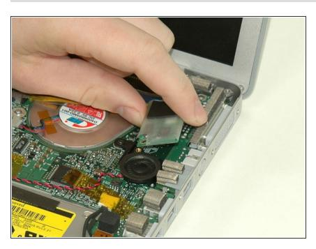
Lift the right ambient light sensor board Straight up from the Logic Board.
