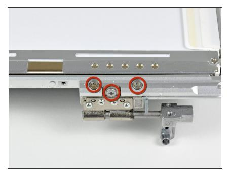
Remove the three T8 Torx screws securing the left clutch hinge to the front bezel.
