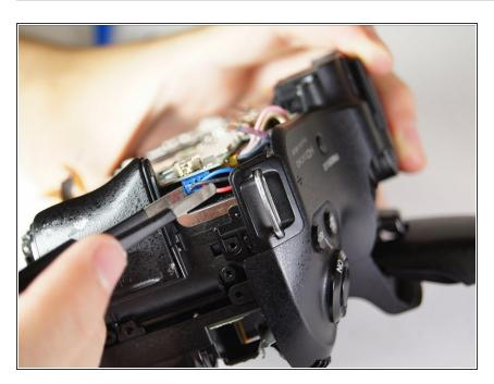
Use tweezers to unplug the blue adapter located at the top right of the circuit board.
