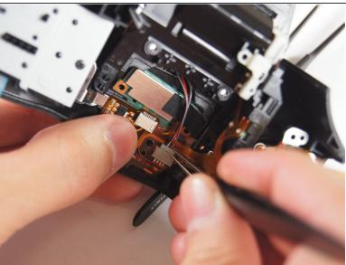
Slowly disconnect the wire from the board using your hands or with tweezers. It may take some wiggling. Try pulling from both sides to disconnect the wires more easily.
