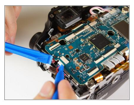
Use either plastic opening tools or tweezers to unplug the white adapter located on the right side of the circuit board.
