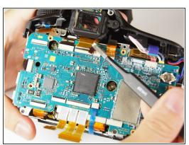
Use tweezers to disconnect the blue, gold, and brown ribbon connectors near the top of the camera.
