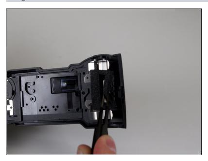
Use the <u>tweezers</u> to carefully peel back the adhesive foam connecting the back panel to the case and remove the panel.
