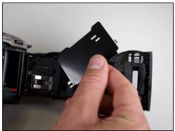
• Remove the black case by gently lifting it with your fingers and rotating counterclockwise.
