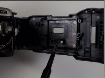
• Use the tweezers to carefully peel off the rubber clock button.
