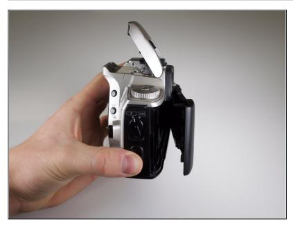
Open the back panel by firmly pressing up on the back-cover release on the lower right side of the camera.
