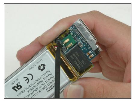
Use a spudger to scrape away the black glue covering the three battery wires.
