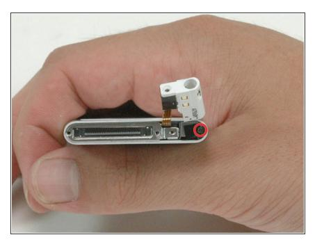
Remove the newly-revealed Phillips #00 screw from beneath the headphone jack. Be careful, this screw is easily stripped.
