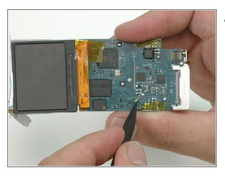
Bend the wires over to prevent them from sliding out of the logic board.
