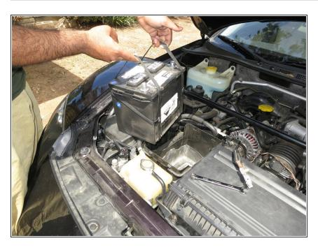
After removing the bar pull the dead battery out using the black straps.
