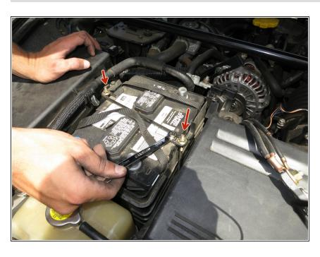
Using the 10mm Wrench remove gold nuts that hold the retention bar in place.
