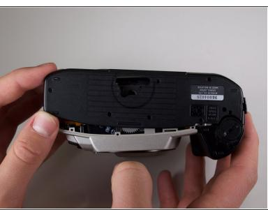
Remove the seven black Phillips #00 5.0 mm screws from the bottom panel. The bottom panel is now free to come off.
