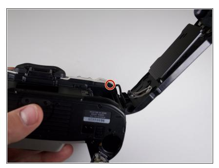
Remove the black Phillips #00 4.0 mm screw from the inside top right section of the camera.
