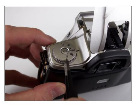
Using the tweezers, remove the dial from the top of the camera.
