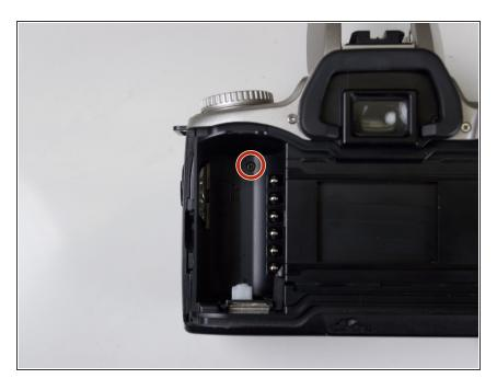
Remove the black Phillips #00 5.0 mm screw from the back of the film compartment.
