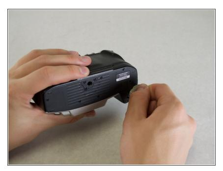
Use the edge of a coin to twist open the battery compartment on the bottom of the camera. (Twist counterclockwise)
