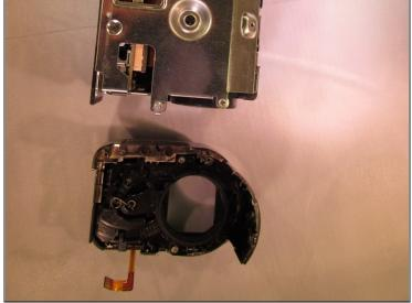
• Pry upwards on the front cover from the top of the device and with your other hand pull straight out on the front of the device (The front cover will be detached and free).
