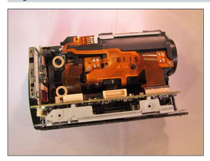
Locate the two black 4 mm screws located on the inside of the device and unscrew them.
