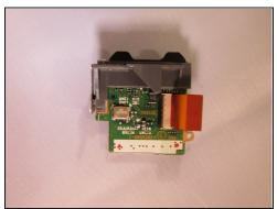
• Pull the SD card slot slightly to the side and detach the SD card slot (the SD card slot is ready to be replaced).
