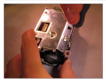
Remove the 6 mm screw on the top of the metal casing which was under the front cover.
