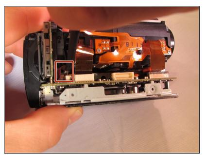
• Disconnect the ribbon cable on the back of the SD card slot.
