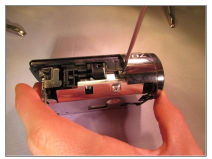
• Unscrew the silver 4 mm screw from on top of the camcorder.
