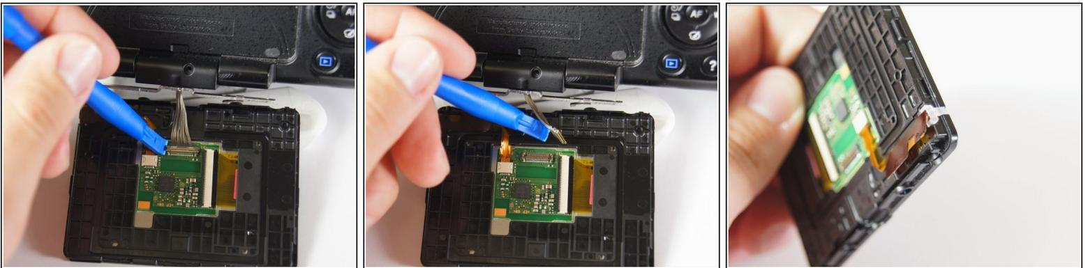
**⚠** The brown ribbon and white light on the edge of the screen are extremely loose and will fall off. Keep the screen flat at all times to make sure they don't come out.
