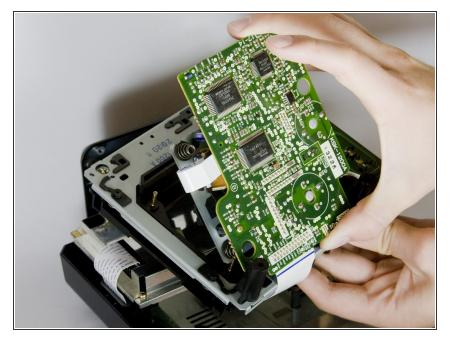
• Carefully remove the CD tray from circuit board.
