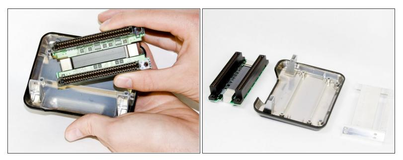
• Remove the connector from the housing.
