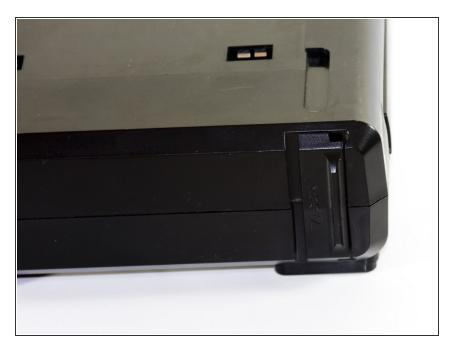
• Slide the lock tab to the left to separate the halves of the console.
