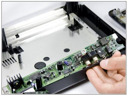
• Remove the power supply unit from the console by lifting the unit up.
