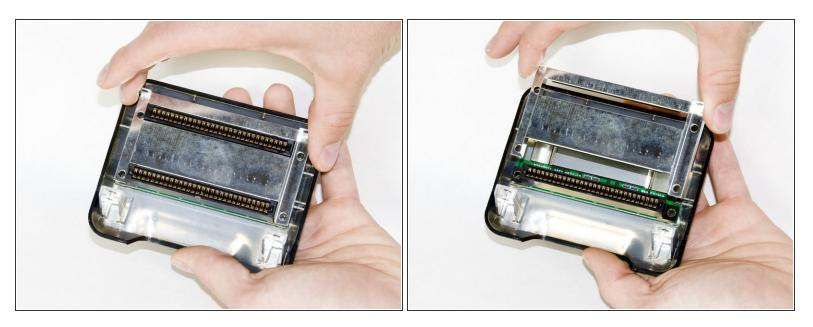
• Carefully remove the metal cover from the connector by sliding the cover up and out.
