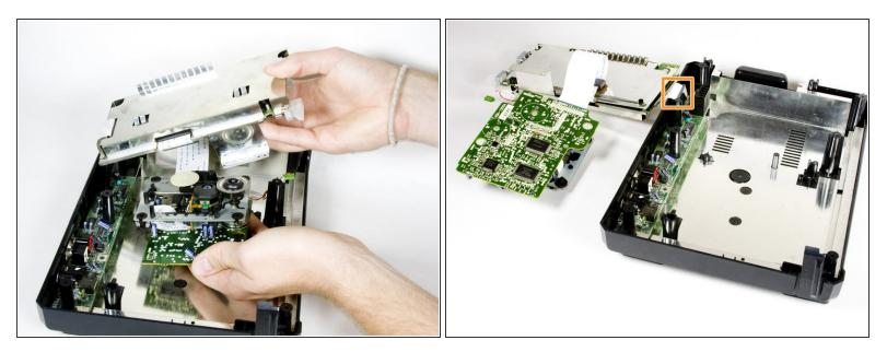
• Carefully lift off the metal plate, the motherboard, and the CD tray circuit board. Then, flip each piece over, as pictured.
