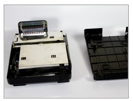
• Lift the top of the case to remove the cover.
