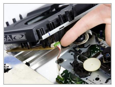
• Carefully unplug the wire connected to optical reader.
