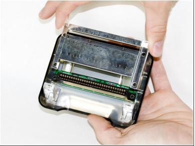
Carefully remove the metal cover from the connector by sliding the cover up and out.
