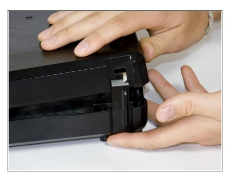
Lift from the left side to remove the top of the case.
