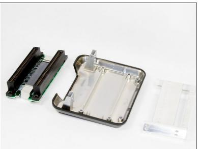
Remove the connector from the housing.
