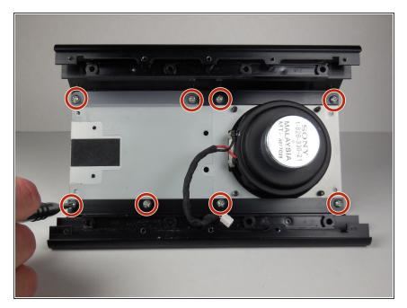
Remove eight 8 mm Phillips #2 screws holding the subwoofer tray to the housing.
