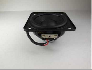
The subwoofer has now been removed from the device and can be replaced.
