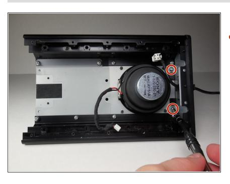
Remove two 8 mm Phillips #2 screws holding the side panel in place.
