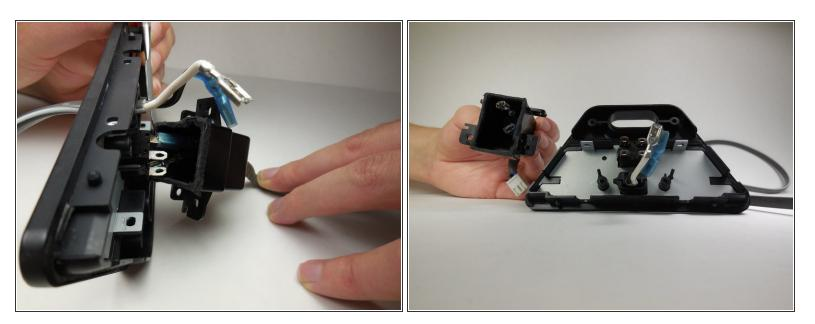
Using a metal spudger, disconnect the four spade connectors that are connected to the power button and the power cord.
