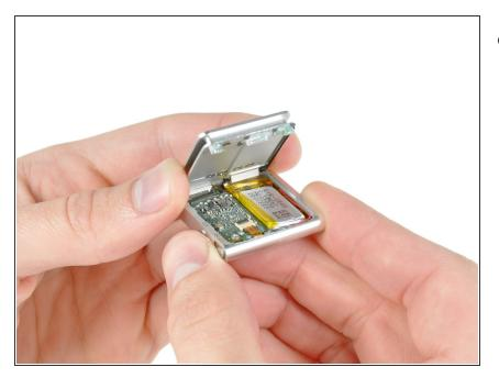
• Remove the rear panel from the Shuffle.
