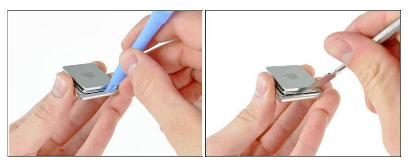
Use a combination of iPod opening tools and metal spudgers to pry the rear panel away from the Shuffle by the seam nearest the ON/OFF switch.
