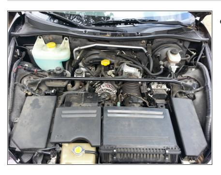
Remove the plastic engine cover by lifting up.
