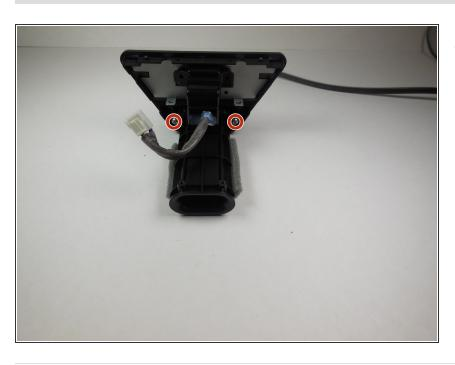
The subwoofer air tunnel can be removed by unscrewing the 2 XXXX screws with a Phillips #2 screwdriver.
