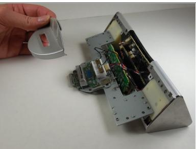
Remove the plastic dock cover by using two fingers to push the attached metal piece forward and slide it out of the holes.
