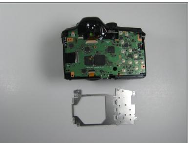
After loosening the frame with the opening tools, gently remove the frame from the interior of the camera.
