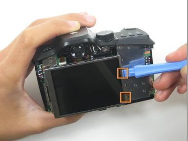
Begin by using Plastic Opening Tools to remove the LCD Screen from it's interior casing. To do
