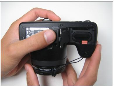
Begin by sliding the switch towards the open symbol. Release your finger from the switch and the battery case will pop open.
