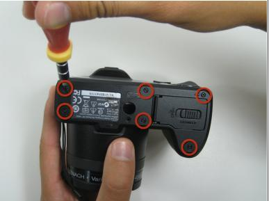
After removing the screws located on the right side, remove the six screws located on the bottom of the camera.
