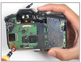
Begin by unscrewing all four screws found in each corner of the frame
