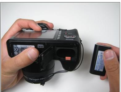
Once the battery has popped out of the compartment, simply pull it out of the camera.
