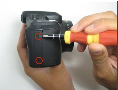
Next, remove the two screws located on the right side of the camera.
