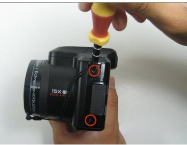
Lastly, remove the two screws located on the left side of the camera.
