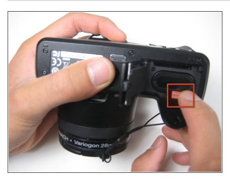
Next, press down on the red lever which holds the battery in place.
