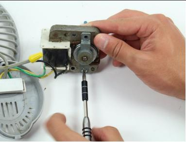
Unscrew the two adjacent motor cage screws to free the motor
