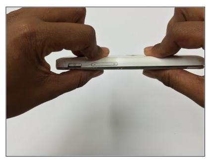
Now put the rear housing cover on the device, starting from its bottom side, and snap the edges all the way around to close the device.
