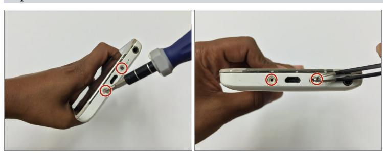
Continue to unscrew the two 10mm Phillips Screws from the bottom of the device.
