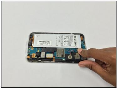
• Insert the battery into its position, and reconnect its tab onto the motherboard.
