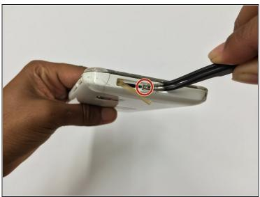
• Remove SD Memory Card before taking the device apart. Using the screwdriver, remove the 10mm Phillips screw that is near the SD Memory Card port.
