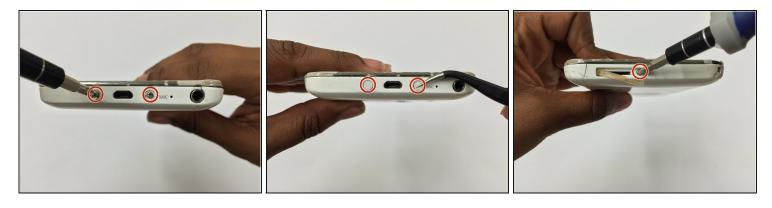
Lastly reinsert the screws at the bottom of the device, as well as the screw inside the SD Memory Card port.
