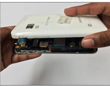
Take the back housing cover off of the device.
