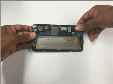
• Gently put in the new rear facing and front facing camera and snap the tab back onto the motherboard.
