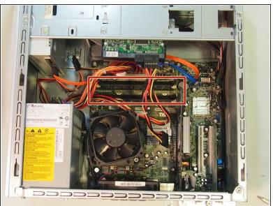
Locate and unscrew the two large screws at the back of the computer. Once the screws are removed, the panel on the right side will slide towards the back, and release itself. Lift the panel off the computer to reveal the internals.
