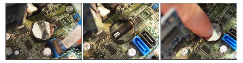
The CMOS battery has to be removed properly to avoid damaging the motherboard.
