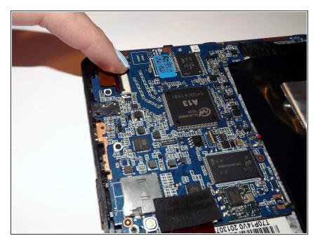
Flip the black latch over the gold cable to the upright position in order to release the cable.
