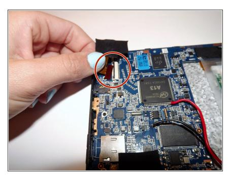
Carefully remove the cable from the circuit by pulling it straight out.
