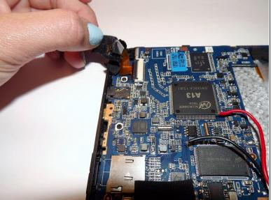
Gently remove the black tape covering the camera and circuit board. The tape will be connected to a foamy block on the back of the actual camera component.
