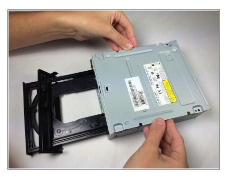
Remove the bottom plate by lifting it off the device.
