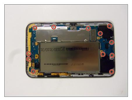
Using the Phillips #00 precisions screwdriver, remove the 12 4mm screws holding in the motherboard.
