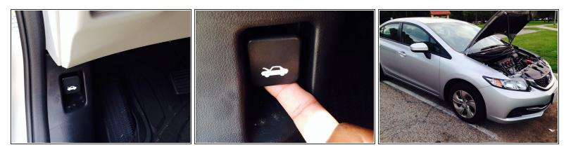
• Locate the "hood open" lever on the driver's side of the inside of the car, below the dashboard. Pull lever toward you. You will hear a "click." Go to the front of the car. The hood should be "popped" slightly. Reach under the hood, find a lever, and move the lever to the left. This will completely release the hood latch.
