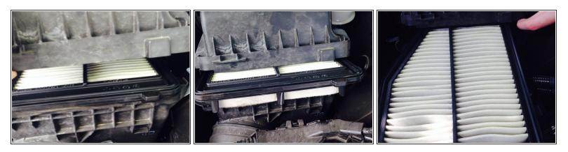
• Gently lift the cover of the box from the lower part of the box. Remove the old air filter from the box and set it aside. Place the new air filter in the box. Replace the cover and place the four clips back on the box.
