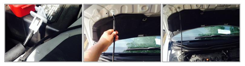
• Find the anchor to hold up the hood of your car. This anchor should be laying along the ledge in front of the radiator. Lift the anchor and insert the end into the hole on the lower side of the hood.
