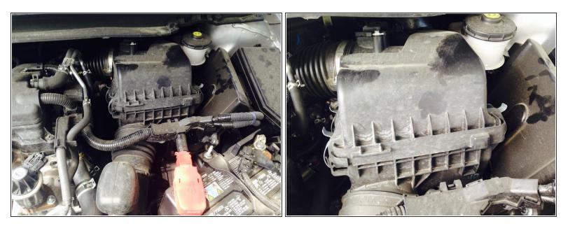
• As you are facing the Civic, the air filter will be inside the black plastic box to the right of the valve cover.
