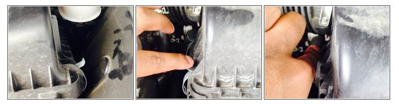
• There will be four clips on the air filter box - two on the front, one on the right and one on the right back. Release the clips from the box by pushing them away from the box.
