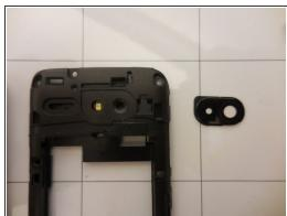
• Use the spudger to pry the camera lens and remove it from the rear frame. Then you can replace the lens.
