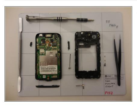
Use the screwdriver with the Y0 bit attached to take out the seven 5mm screws that attach the back cover on the phone. Make sure to keep track of these screws, as they are pretty important.
