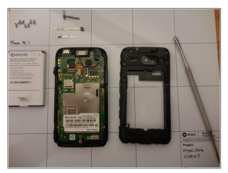
Next, use the metal spudger to pry at the plastic clips. Be careful to not to lose the power button and volume buttons as they fall out. Remove the plug for the camera flash.
