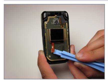
Using a plastic opening tool, lift the ribbon cable connection below the front LCD.
