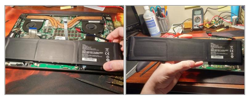
Remove the battery by pulling up from the side closest to the motherboard
