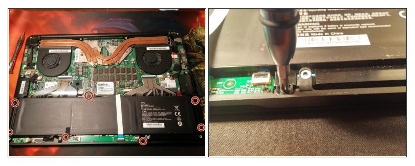
Remove the 7 battery screws
