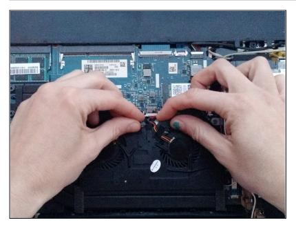
• Carefully pull out the small white plug connecting the fan to the motherboard.
