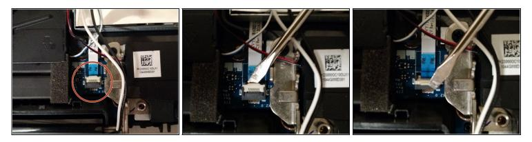
Use a small flathead screwdriver to pull upwards on the tab connecting the white ribbon wire to the board. Unhook the white wire from the black latch.
