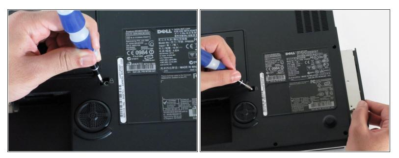
• Use the screwdriver to gently push the optical drive out
